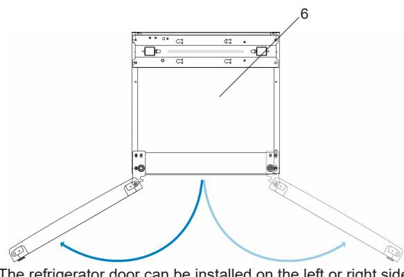
The refrigerator door can be installed on the left or right side.
